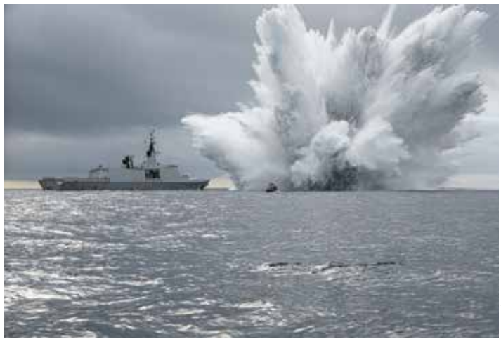
Impact tests on refitted light frigate Courbet – 2025.
