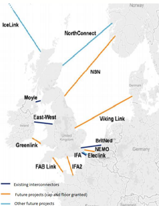
Figure 1. Map of existing and planned interconnectors between the UK and neighbouring countries (Initial source: Pöyry, 2016)
